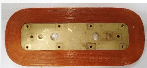
Double Pancake Coil with Vacuum Pressure Impregnation
